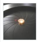
Integrating a consistent and powerful 30W Quartz Halogen Bright field illumination with a precise, adjustable aperture diaphragm [Ø41mm - Ø2mm], you are able to measure with a table gauge the proportions and pavilions of a diamond.
